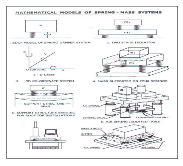
For slowest Operating speed = 500 rpm Vertical isolation efficiency > 98% System natural frequency = 1.8 Hz. Applications are in laboratories and ground transportations only. Example-Vibration Isolated Table.
